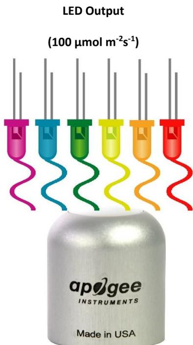
Example of photon flux density measurement with an Apogee model SQ-644 Quantum Light Pollution Sensor. The LED in this example Full yields a photon flux density on a horizontal plane of  $100 \mu\text{mol m}^{-2} \text{s}^{-1}$ . This yields an output signal of 12 mA. This signal is converted to photon flux density by subtracting the 4.0 mA offset and then multiplying by the calibration factor of  $12.5 \mu\text{mol m}^{-2} \text{s}^{-1} / \text{mA}$ .
