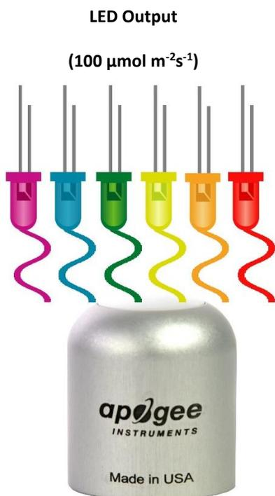
Example of photon flux density measurement with an Apogee model Quantum Light Pollution Sensor. The LED in this example Full yields a photon flux density on a horizontal plane of  $100 \mu\text{mol m}^{-2} \text{s}^{-1}$ . This yields an output signal of 1250 mV for the 0-2.5 V option or an output signal of 2500 mV for the 0-5 V option. This signal is converted to photon flux density by multiplying by the calibration factor.
