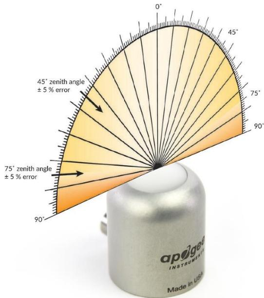
Directional, or cosine, response is defined as the measurement error at a specific angle of radiation incidence. Error for Apogee SQ-600 series Quantum Light Pollution Sensor is approximately  $\pm 2\%$  and  $\pm 5\%$  at solar zenith angles of  $45^\circ$  and  $75^\circ$ , respectively.
