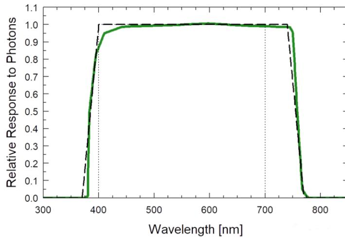
Mean spectral response measurements of four replicate Apogee SQ-600 series ePAR Sensors. Incremental spectral response measurements were made at 10 nm increments across a wavelength range of 370 to 800 nm in a monochromator with an attached electric light source. Measured spectral data from each quantum sensor were refined and normalized by comparing measured spectral response of the monochromator/electric light combination to measured spectral differences from a quantum sensor reference.
