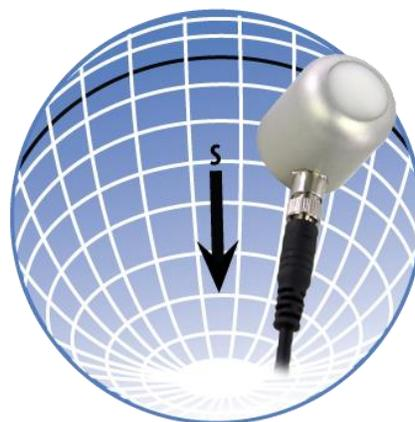
In addition to orienting the cable to point toward the nearest pole, the sensor should also be mounted such that obstructions (e.g., weather station tripod/tower or other instrumentation) do not shade the sensor. **Once mounted, the blue cap should be removed from the sensor.** The blue cap can be used as a protective covering for the sensor when it is not in use.
