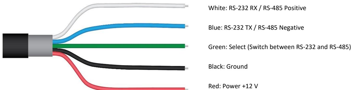
The Green wire should be connected to Ground to enable RS-485 communication, or it should be connected to 12 V power for RS-232 communication. Text for the White and Blue wires above refers to the port that the wires should be connected to.
