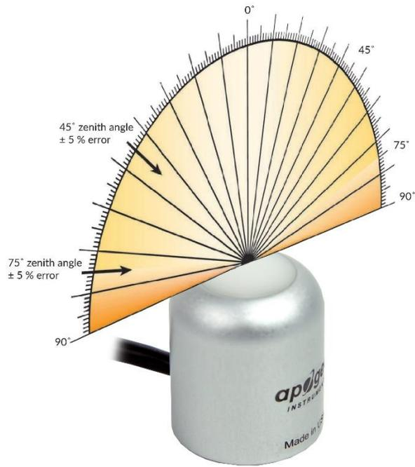
Directional, or cosine, response is defined as the measurement error at a specific angle of radiation incidence. Error for Apogee SQ-600 series ePAR Sensor is approximately ± 2 % and ± 5 % at solar zenith angles of 45° and 75°, respectively.
