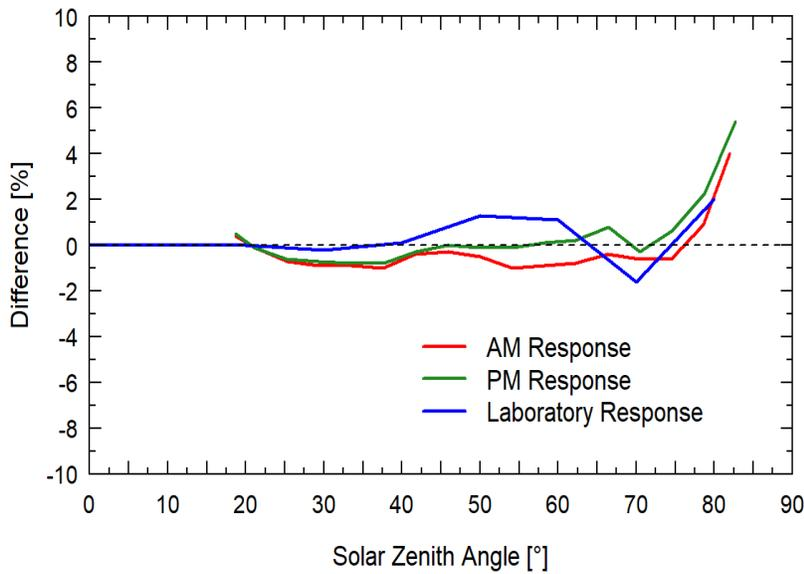
Mean directional (cosine) response of seven Apogee series quantum sensors. Directional response measurements were made on the rooftop of the Apogee building in Logan, Utah. Directional response was calculated as the relative difference of quantum sensors from the mean of replicate reference quantum sensors (LI-COR models LI-190 and LI-190R, Kipp & Zonen model PQS 1). Data were also collected in the laboratory using a reference lamp and positioning the sensor at varying angles.
